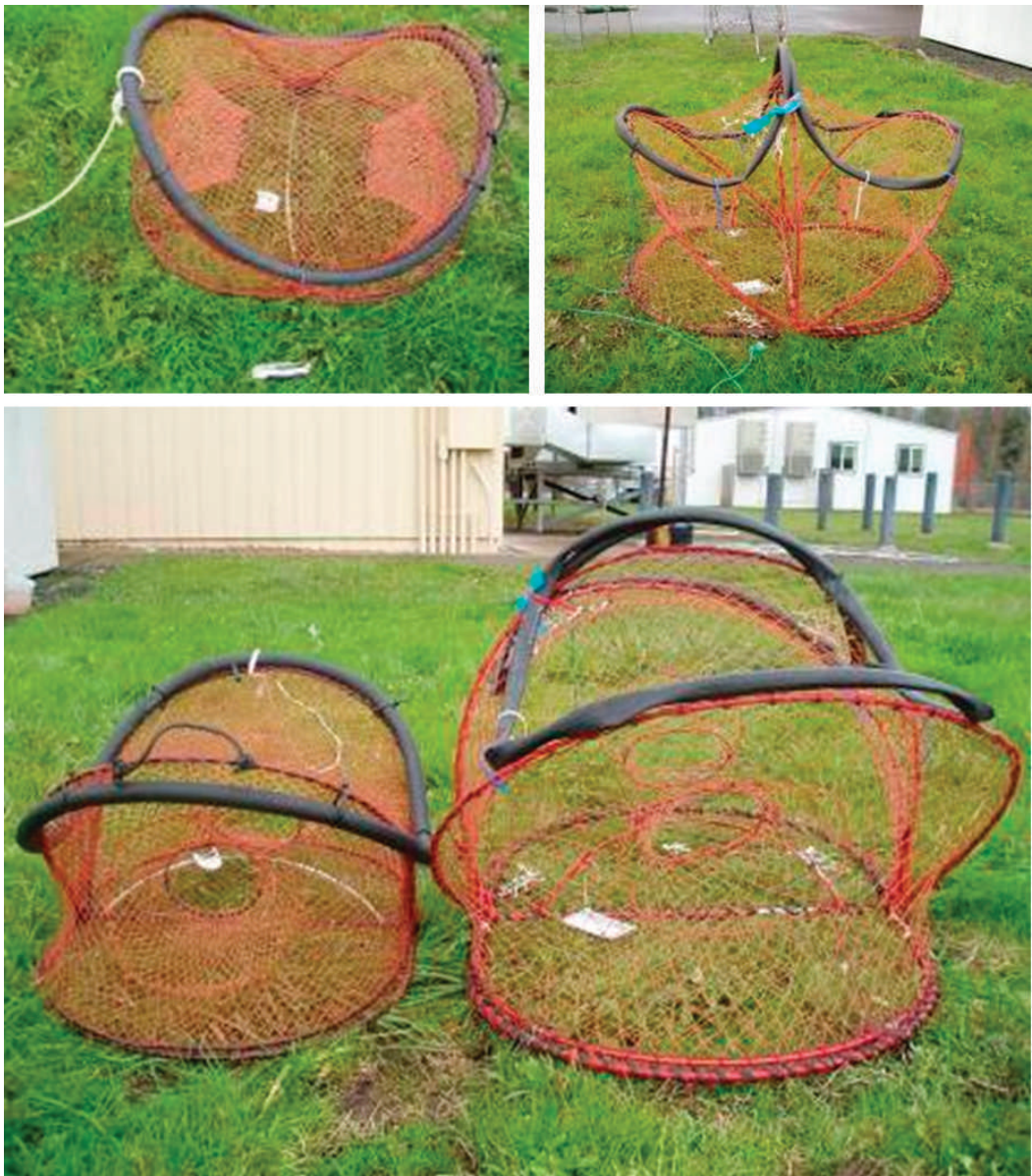
FIGURE 12. Commercial collapsible traps. Top Left: View of a moderate sized trap that is lightweight and portable. Top Right: Side view of large version. Bottom: Side-by-side comparison of mouth and funnel of traps. Bicycle inner tubes tied around outside of traps serve as floats (air added when in field). White twine on large trap shows areas where we mended traps in field.
